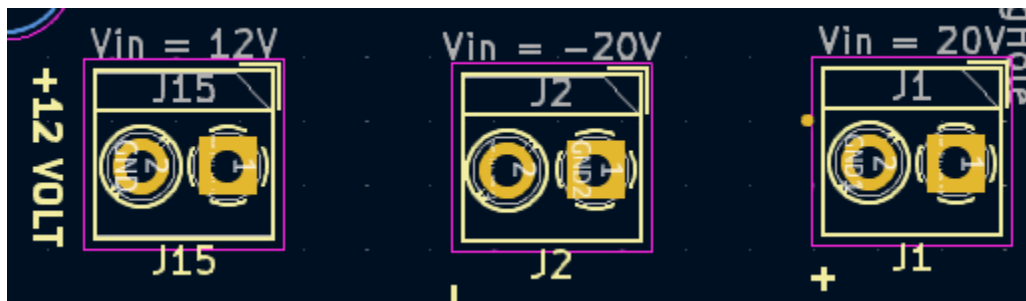
Figure: +20, -20, and 12V input in the current prototype
